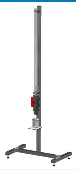
The FL 14.3 equipment is designed to determine in a quickly and easy way the dynamic viscosity of a fluid.
